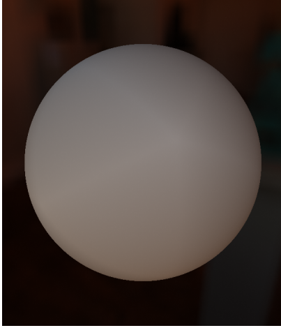
Figure 4: Mach bands visible when linear interpolation is used between icosahedron vertices
